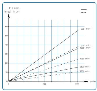
Cut item length is achieved by selection of cutter type with 2 or 3 blades and choice of motor speed. Strip speed must be known. Cut item length can vary. The lengths stated are examples.
